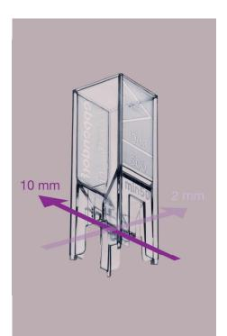
The patented\* Eppendorf UVette is a fully UV-transparent, single use cuvette made of clear plastic, with a light transmission of 220 nm to 1,600 nm. The unique design allows you to conduct flexible measurements with two different light paths (10 mm and 2 mm).
