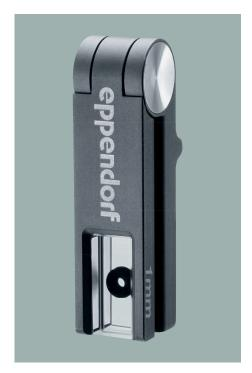
With an optical path length of only 1 mm, the  $\mu$ Cuvette G1.0 features a light path that is ten times shorter than the light path on standard cuvettes. This allows high nucleic acid and protein concentrations to be measured using the  $\mu$ Cuvette G1.0. Only 1.5  $\mu$ L of a sample is required for the measurement. The  $\mu$ Cuvette G1.0 offers a flexible expansion of the photometric application range of Eppendorf photometers.
